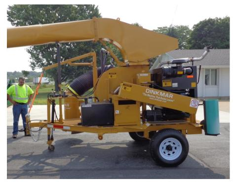
Pictured above is maintenance supervisor Matt Seamon as he inspects the township's new leaf vacuum. It was purchased to replace the old vacuum which was acquired, used, in 2004. The new machine is equipped with a hydraulic vacuum arm controlled by an operator riding at the back of the machine. The new equipment will have a longer reach than the machine it is replacing.
